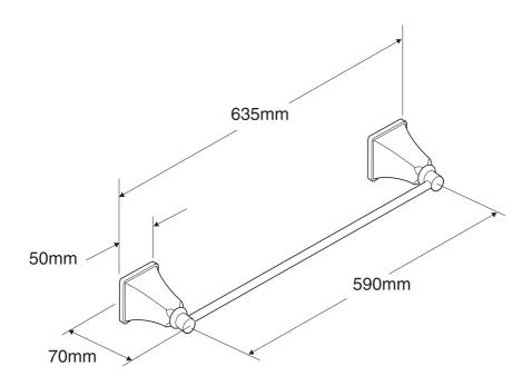
All measurements shown are in millimetres. Sizes are approximate.
